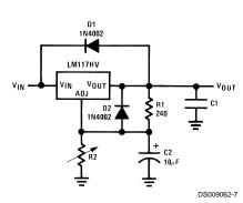
FIGURE 3. Regulator with Protection Diodes
