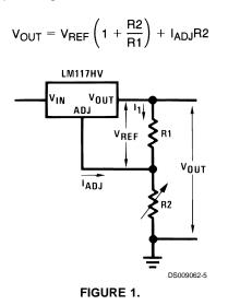
Since the 100  $\mu$ A current from the adjustment terminal represents an error term, the LM117HV was designed to minimize I<sub>ADJ</sub> and make it very constant with line and load changes. To do this, all quiescent operating current is returned to the output establishing a minimum load current requirement. If there is insufficient load on the output, the output will rise.
