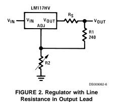
With the TO-3 package, it is easy to minimize the resistance from the case to the set resistor, by using two separate leads to the case. However, with the TO-5 package, care should be taken to minimize the wire length of the output lead. The ground of R2 can be returned near the ground of the load to provide remote ground sensing and improve load regulation.
