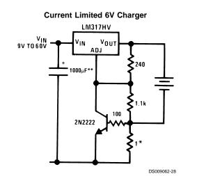
\*Sets peak current (0.6A for 1Ω) \*\*The 1000  $\mu F$  is recommended to filter out input transients
